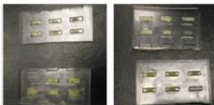
Figure 3. Films have been fabricated in Cady B (Left) and Cady Bv2 (Right). The yellow dye was added to visualize the films clearly. After drying for two days, the films were ready for release study.
