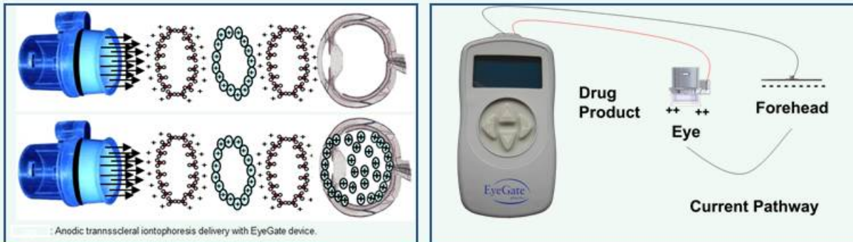
: Anodic transscleral iontophoresis delivery with EyeGate device.
